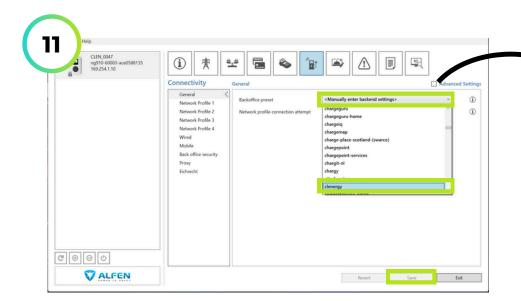
11. In the Backoffice preset field, select Clenergy from the drop-down menu. Then select Save and allow the charge point to reboot. In the Network profile connection attempt field, it is recommended to reduce the number to 1.
