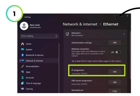
1. Use a RJ45 Ethernet cable to connect your device to the charge point. Please ensure your IP Assignment is set to Automatic (DHCP) as highlighted.
